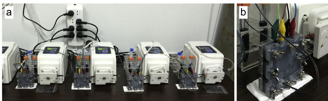
Fig. 1. (a) Experimental setup for VFB battery performance evaluation. (b) A close look of the VFB single cell.
